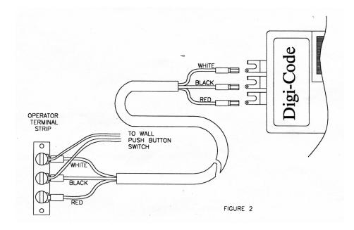
Slip on connectors at one end of the adapter connect to the flat side of each spade lug on the receiver, and the spade connectors at the other end connect to the operator terminal.
