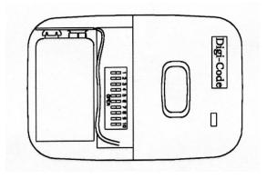
**Set both code switches to the code of your choice**, being sure both are set the same since a different setting of just one switch will prevent operation. The digital code is determined by the position of the 10 small switches numbered 1 through 10 located in the receiver and the transmitter. Any combination of "on" or "off" positions can be selected by using a pencil or a pen. (Note: The switches are in the "on" position when the switch is depressed toward the number.) See Figure #3 above.
