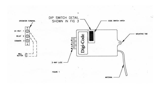
For remote installation the receiver may be mounted near the operator head on a joist or the ceiling by using the mounting tab. Order Model 5192-06 adapter, which permits connection between the operator terminal and the two-way lugs on the receiver.
